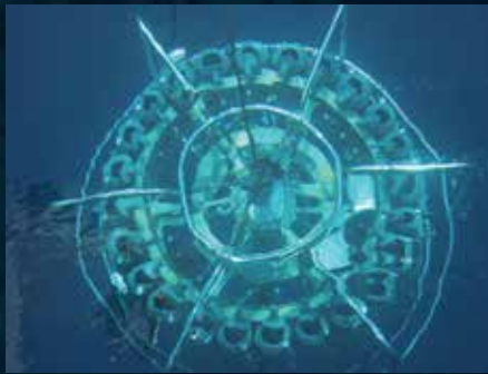
ROSETTE SAMPLER INSTRUMENT USED TO COLLECT WATER SAMPLES
