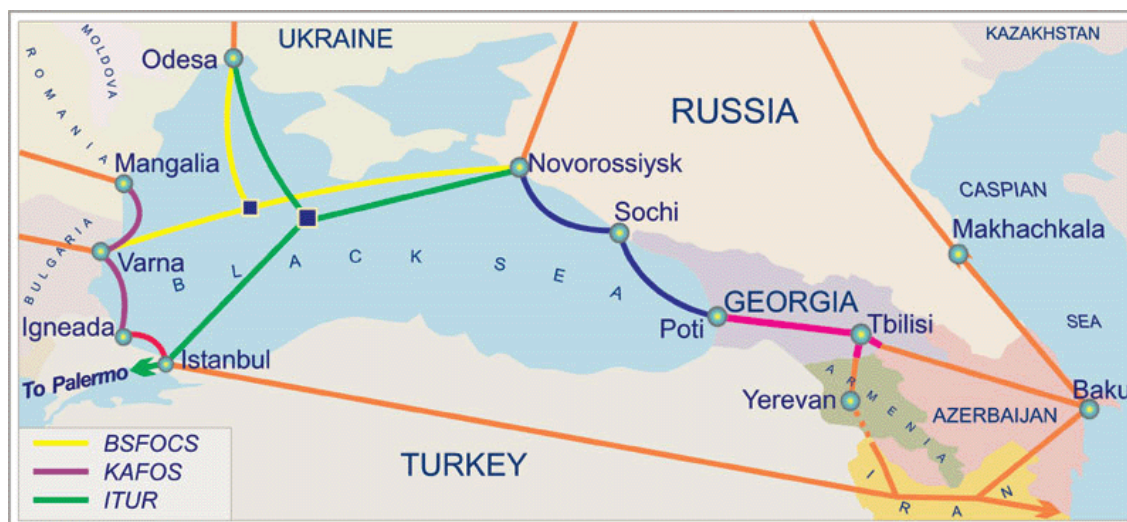
Figure 43. Schematic Map of the Black Sea telecommunication cables.
