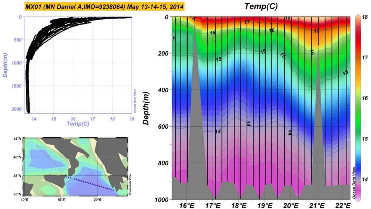
Figure 33. XBT data along MX01 on 13-15 March 2014: Temperature profiles and contour plots, positions of the XBT drops along the transect.
