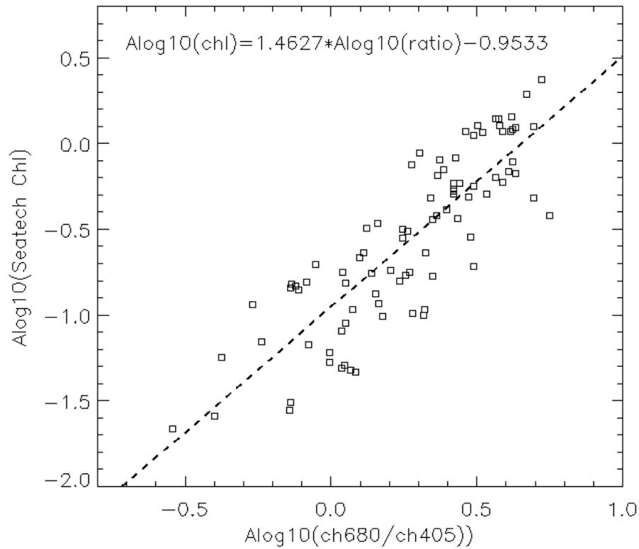
Figure 36. Calibration of the Lidar measurements during BIOOPT 2013 (April 2013).
