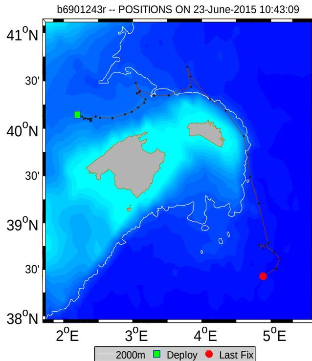
Figure 21. Trajectory and profile positions (black dots) of Apex (WMO 6901243) float deployed by CSIC in the Balearic Sea.
