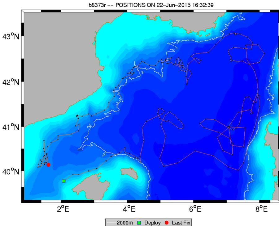
Figure 19. Trajectory and profile positions (black dots) of Apex (WMO 6900786) float deployed by CSIC in the Balearic Sea.
