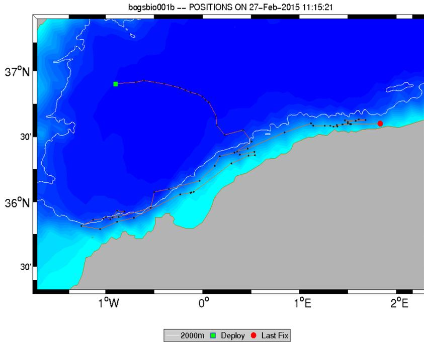
Figure 10. Trajectory and profile positions (black dots) of Provor-BIO (WMO 6901861) float deployed by OGS in the eastern Alboran Sea.
