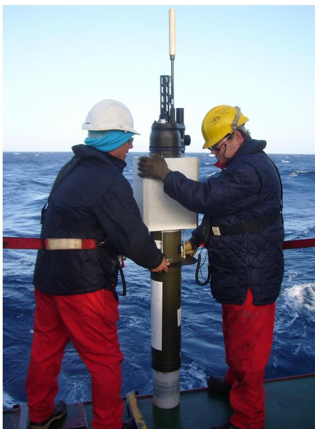
*Figure 12. The Italian Provor-NUT float (WMO 6901865) is ready to be deployed from the R/V OGS Explora in the southern Adriatic Sea on 18 February 2014 during the ADREX campaign.*
