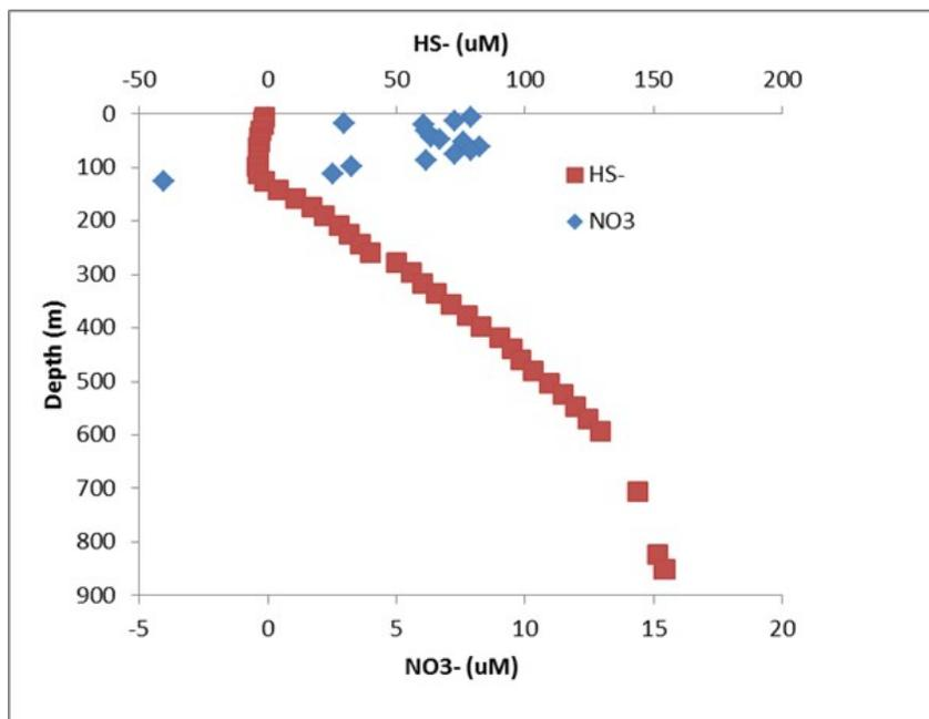
Figure 14. Example of profiles of nitrate and hydrogen sulfide measured by the Italian Provor-NUT float (WMO 6901866) in the western Black Sea.
