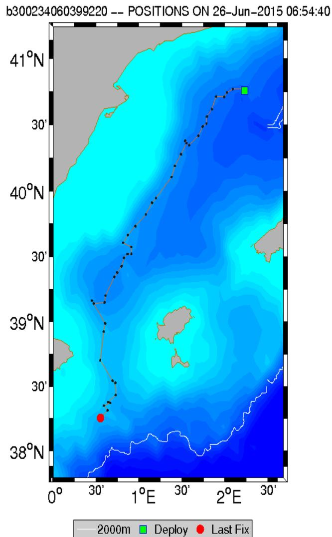
Figure 15. Trajectory and profile positions (black dots) of Arvor-I (WMO 6901245) float deployed by CSIC in the north western Mediterranean.
