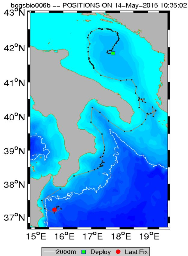
Figure 9. Trajectory and profile positions (black dots) of Provor-NUT (WMO 6901865) deployed by OGS in the southern Adriatic Sea.
