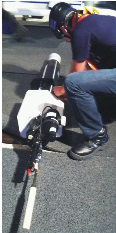
Figure 13. The Italian Provor-BIO float (WMO 6901861) is tested before deployment on the R/V SOCIB in the eastern Alboran Sea on 25 May 2014 during the ALBOREX campaign.
