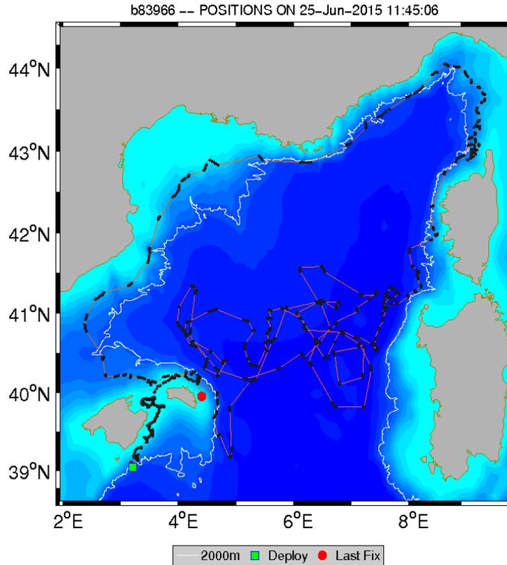
Figure 16. Trajectory and profile positions (black dots) of Apex (WMO 6900662) float deployed by CSIC in the Balearic Sea.
