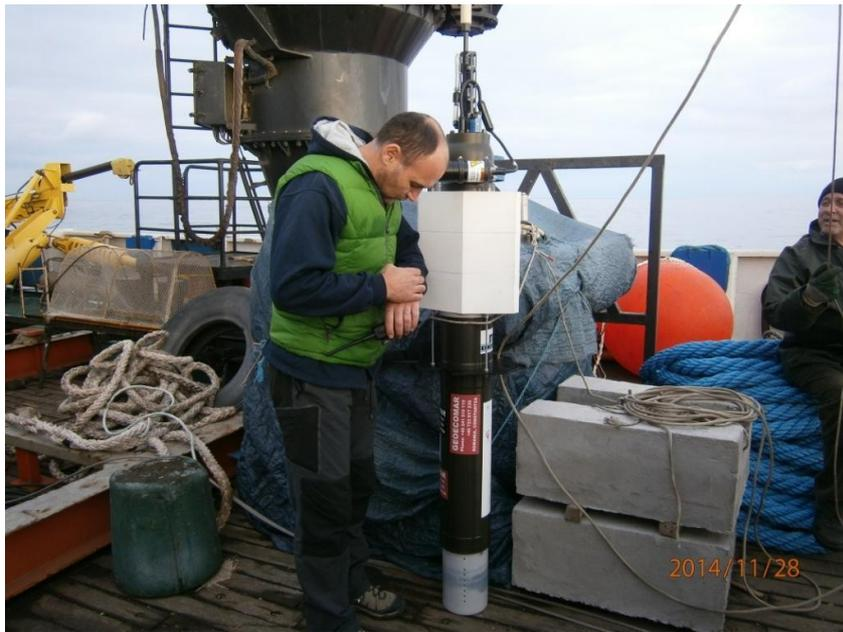
*Figure 3. The Romanian Prov-BIO float is ready to be deployed from the R/V Mare Nigrum in the western Black Sea on 28 November 2015.*
