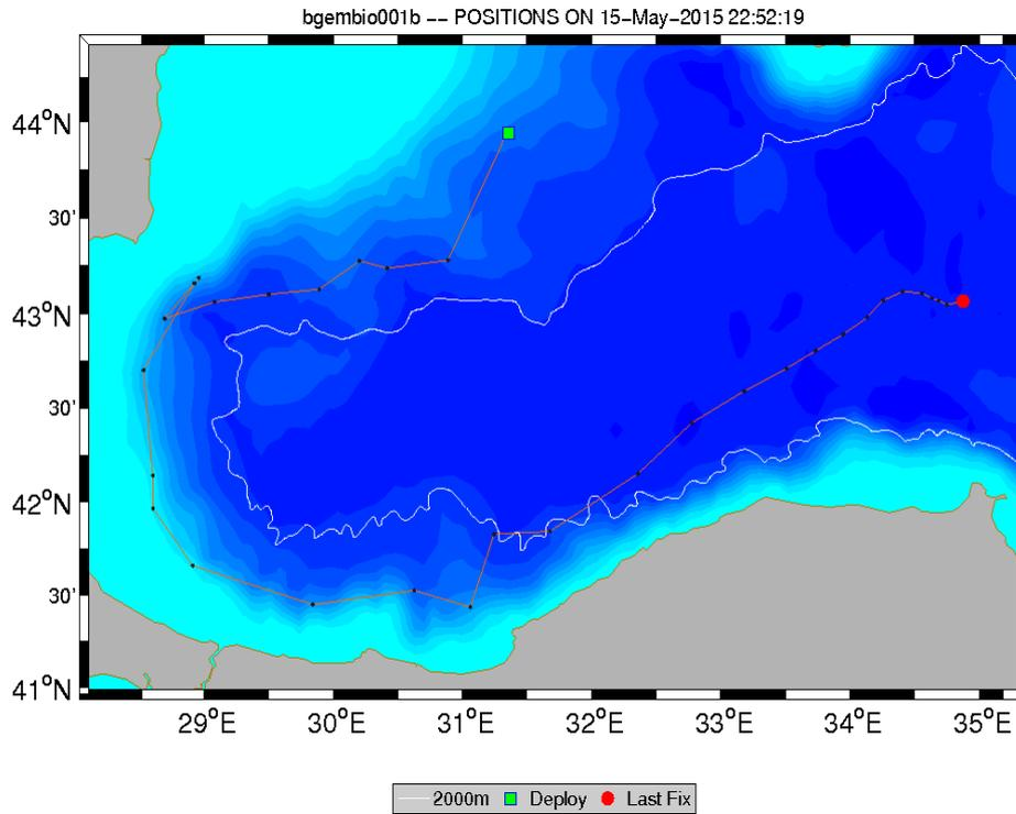
Figure 2. Trajectory and profile positions (black dots) of float deployed by GeoEcoMar (WMO 6900807) in the Black Sea.
