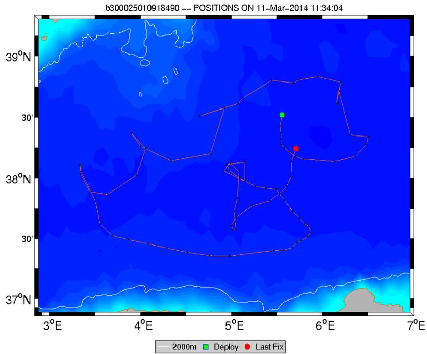
Figure 23. Trajectory and profile positions (black dots) of Provor-BIO (WMO 6901513) float deployed by LOV in the North Western Mediterranean Sea.
