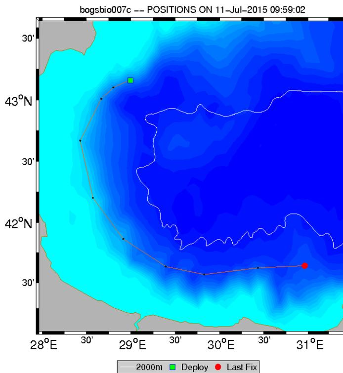
Figure 11. Trajectory and profile positions (black dots) of Provor-NUT (WMO 6901866) float deployed by OGS in the western Black Sea.
