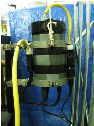
Picture 1. The pCO 2 sensor during the laboratory tests. The pump flushing the internal measuring path is visible on the right. The sensor is installed on its two support brackets that will be used to attach it to the buoy body at 6 m depth
