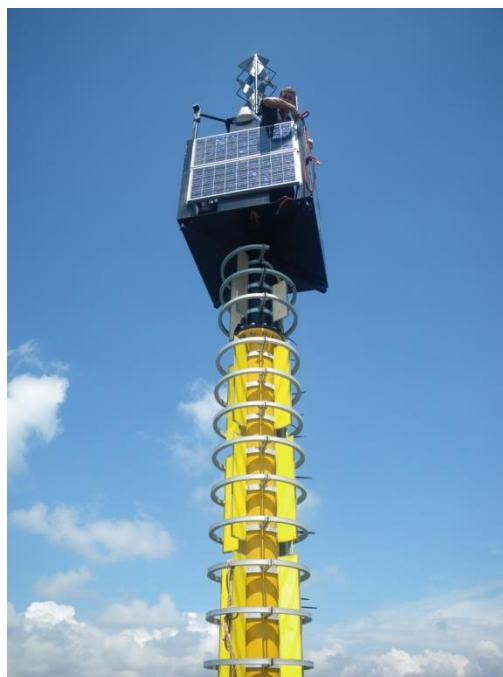
Figure 8. MesuRho observatory instrumentation: meteorological station + PAR (1), ABIN control and transmission (2), multi-parameter probes (temperature, pressure, conductivity, turbidity, fluorescence, dissolved oxygen) (3, 6), ISUS nitrate sensor (4), benthic station (5)
