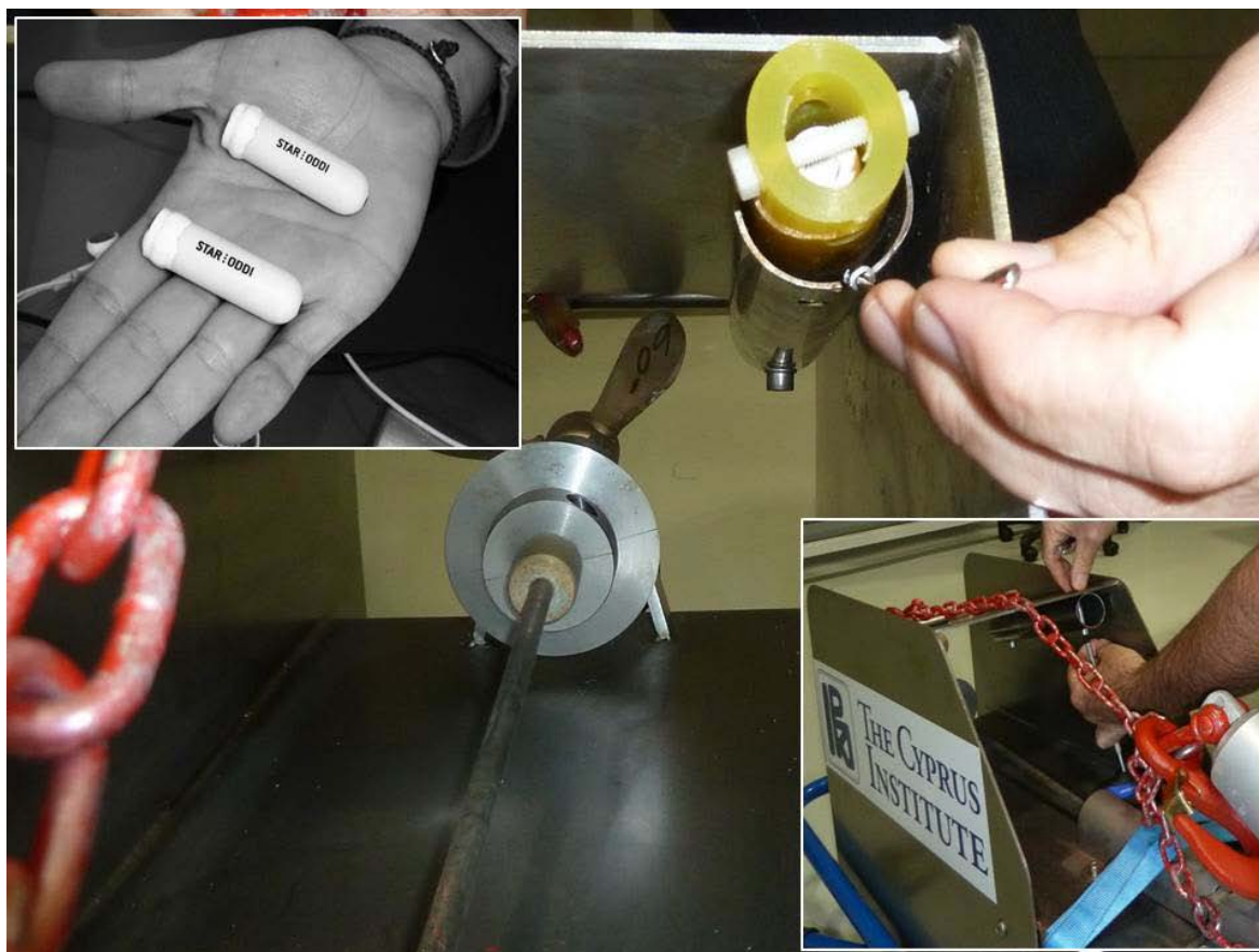
Figure 3: Data logger for temperature, salinity and depth. The logger is installed inside the box double tail fins of the CPR. During the tow, the logger measures once every minute and the data can be referenced according to the position and time of measurement.
