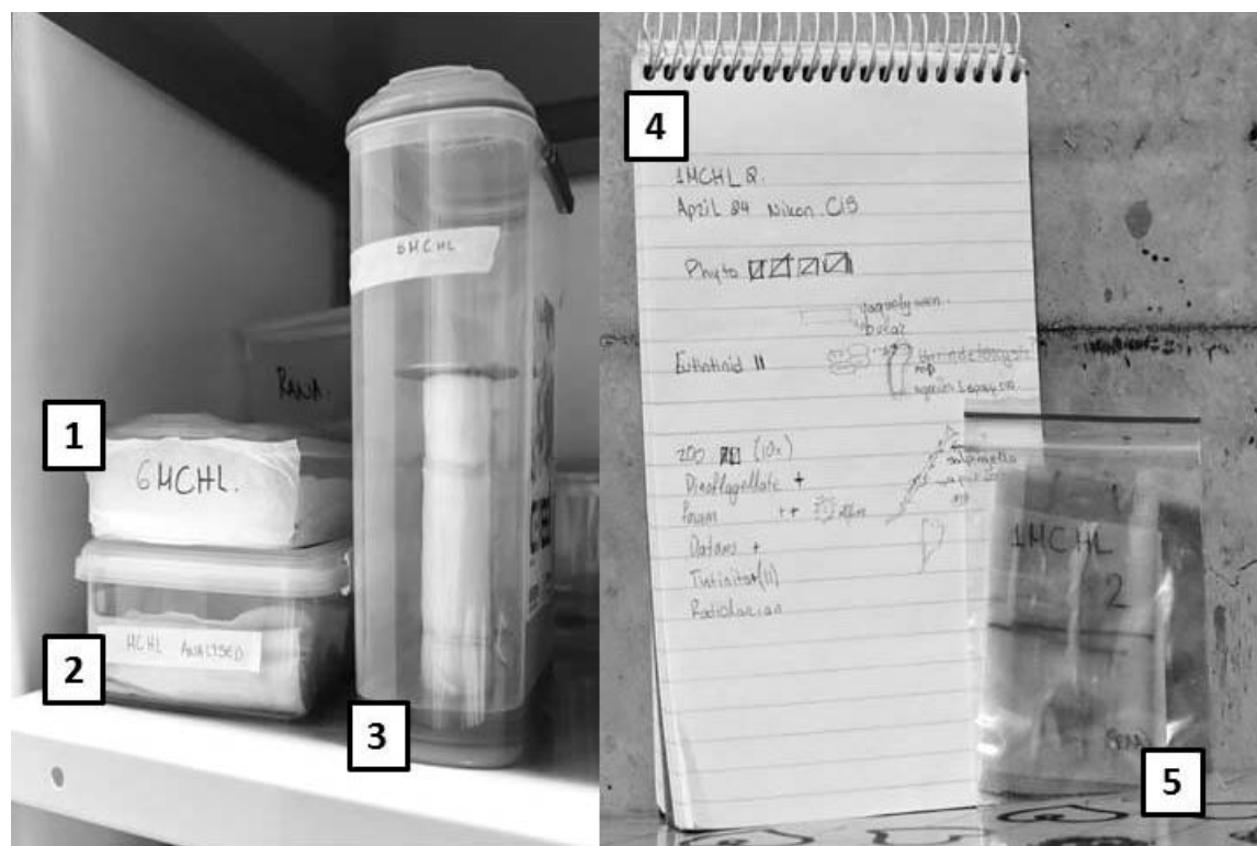
Figure 5: Samples are stored in the MedCPR laboratory in plastic boxes before the analysis [1-2]. The silk holding the sample can also be stored on the spool [3]. When samples are analysed the information is recorded on a notepad [4]. Later each sample is stored in individual ziplock bags.
