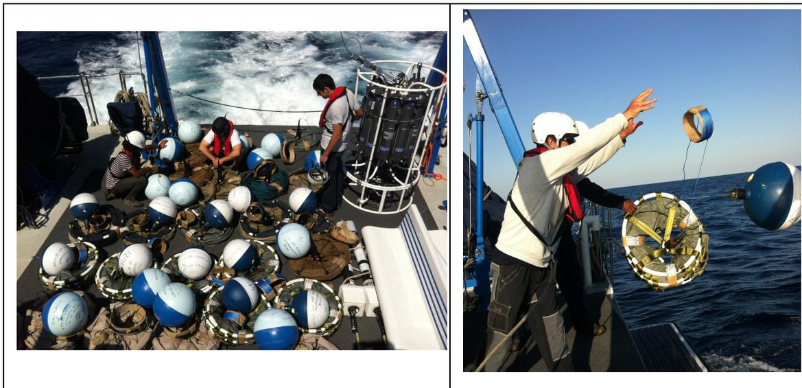
**Figure 18.** Drifter preparation and deployment on board R/V SOCIB.
